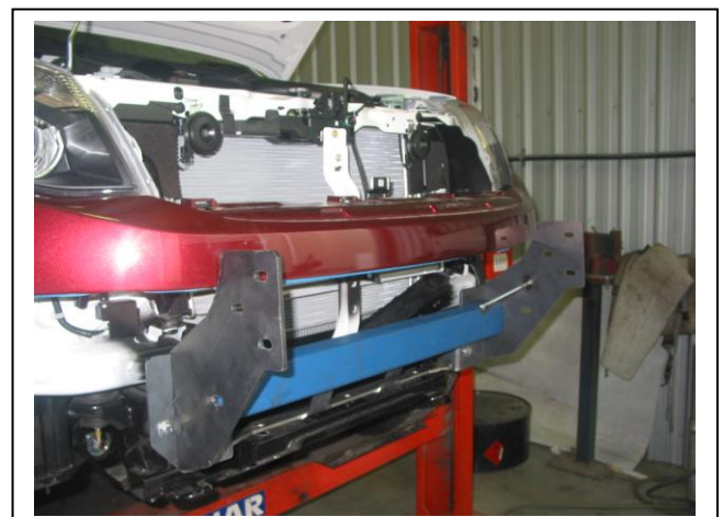
Figure 6: ECB steel mounts with bumper fitted.
